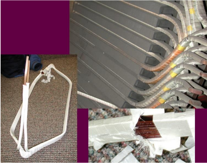
Figure 10 - Form wound insulation.
