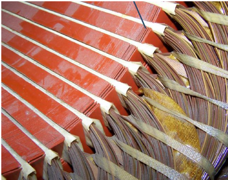
Figure 50 – Older motor with thick laminations.
