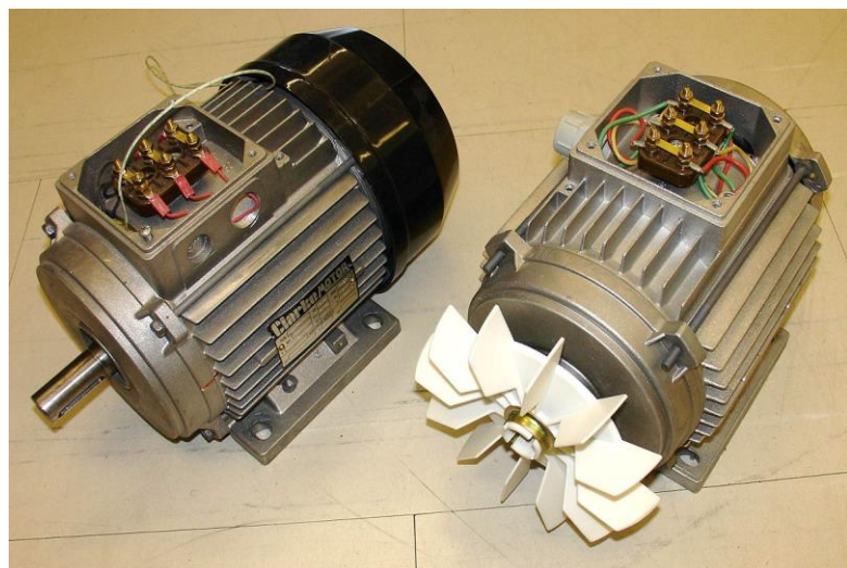
Figure 30-- TEFC motor with fan shroud removed. Picture by Zureks - Pinterest.com
